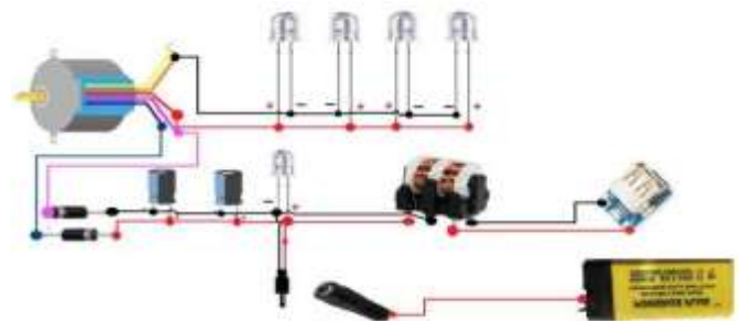
Fig.4.1. Circuit Diagram of Foot Step Power Generation System
